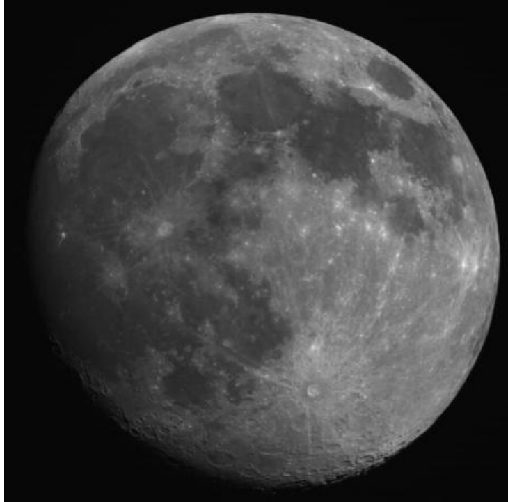
Figure 2. ASTER image of the Moon, acquired 14 April 2003, band 1 (550 nm). The Level-0B1 image has been corrected for the oversampling factor of 4.58 in the down-track direction. Lunar North is approximately 11 o'clock in this figure.
