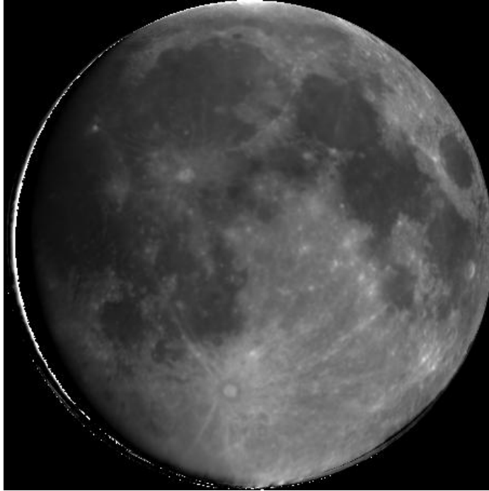
Figure 3. ROLO model radiance image, projected to the perspective of the ASTER lunar view.
