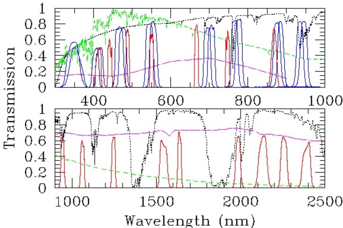
Passbands for the two ROLO telescopes. Common remote sensing bands are shown in red; stellar color pairs are blue. Also shown are the detector quantum efficiencies (purple), nominal atmospheric transmission (black), and a normalized solar spectrum (green).
