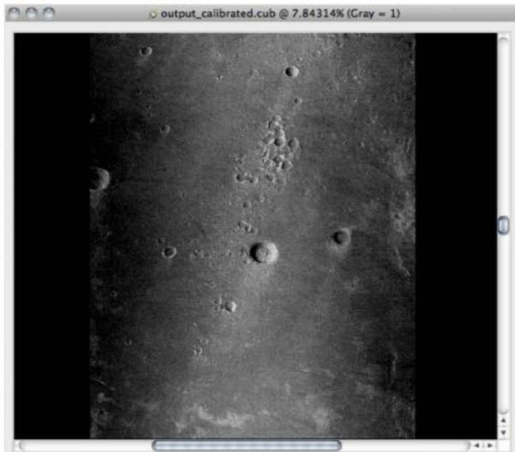
Figure 2: Image P05_003064_1480_XI_32S038W after running pds2isis and ctxcal . Notice the distinct darkening at the image edges.
