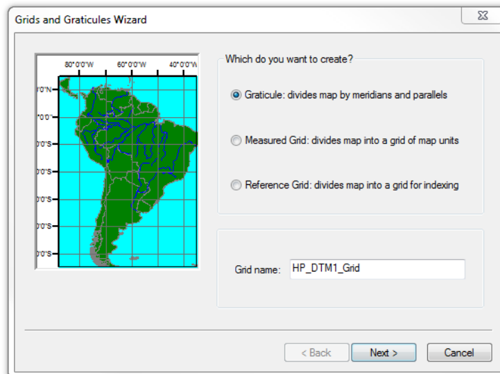
The Grid and Graticule Wizard dialog box – it is helpful to save each with a unique name. The title of this dialog box will change as you progress through the wizard depending on what step you are on.
