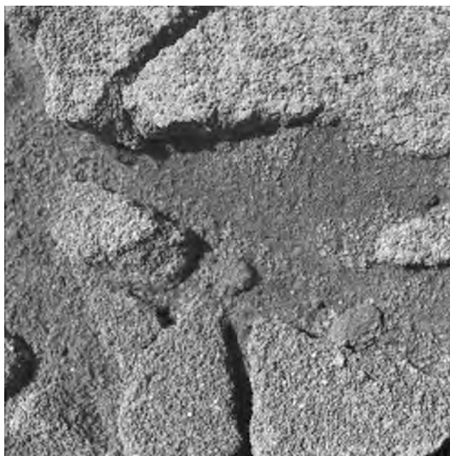
Figure 20.12. Spirit MI image of a disrupted soil crust containing well-sorted 200–300 \mu\text{m} grains, overlying finer material (darker zones in image). Weak soil crusts of varying thicknesses and strengths are common at both MER landing sites. Image 2M170218789IFFAAEEP2976M2F1, obtained on Sol 494 with direct illumination from the upper left, spans about 31 mm.
